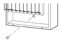
Figure 11 - Installing Bottom Mounting Screw
